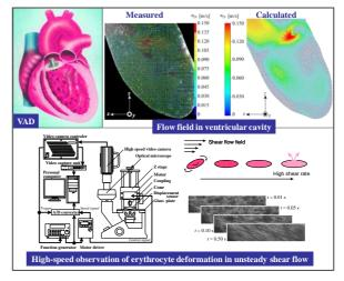
Microscopic high-speed observation of blood cell deformation process in shear flow using microfluidic system
