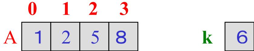
1回目     $left = 0$      $right = 3$      $mid = \left\lfloor \frac{0 + 3}{2} \right\rfloor = \lfloor 1.5 \rfloor = 1$
