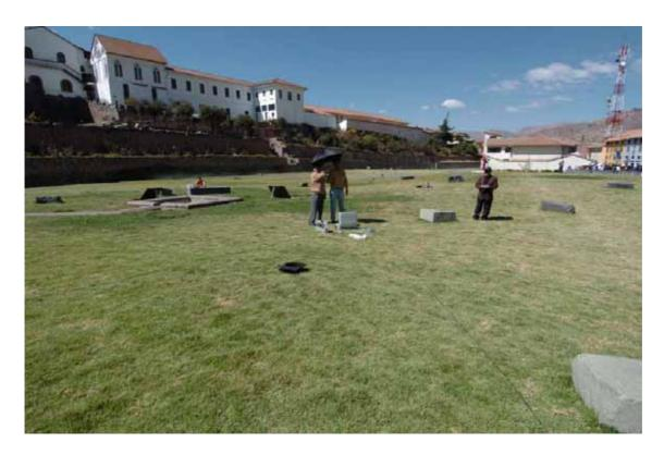
In a manner similar to the interior yard, array measurements of the vertical components of the ground vibration were carried out here. The configuration of sensors again consisted of triangular array with sides of approximately 30 meters as shown in the next figure.
