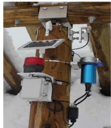
Measurement fence and measurement sensor unit.
