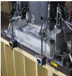
Setup of piezoelectric film sensors
