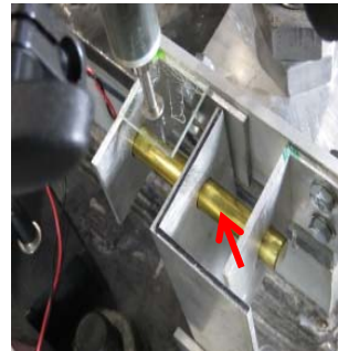
Setup of piezoelectric film sensors
