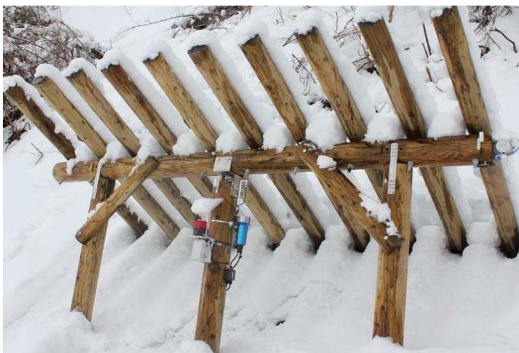
Measurement fence and measurement sensor unit.
