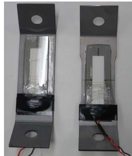
Setting of piezoelectric joint sensor on the steel specimen and SALLY after using sensors.
